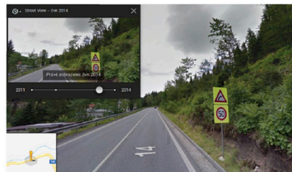
Fig. 7. A hotspot was detected on road segment no. 3639 between 2012 and 2016. It disappeared in all probability as a result of the installation of a warning sign.
